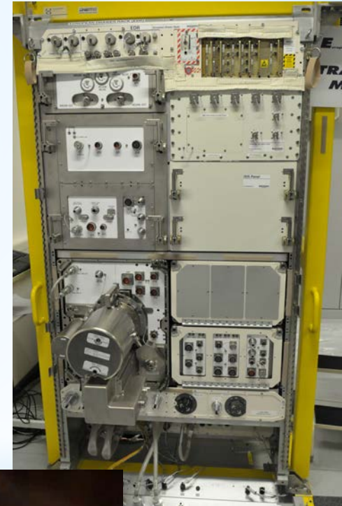
EML Modules inside EDR rack (Training Model)
